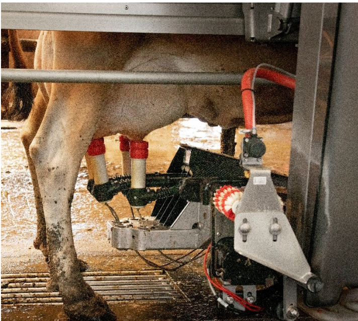
Pictured above is an automated milking system using a robotic milker.
