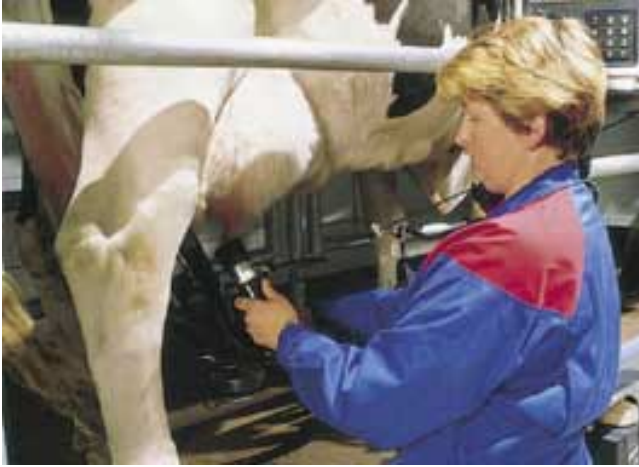
Modern day milking machine shown in use in a milking parlor.
