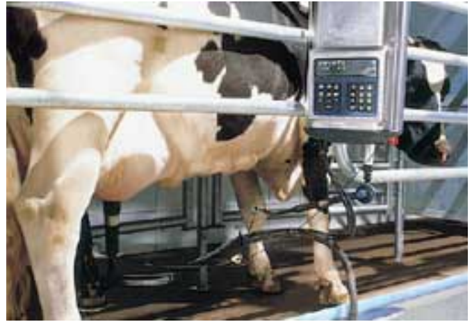
Modern day milking machine shown in use in a milking parlor.
