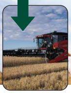
A combine is used to cut the wheat stalk. It also does the threshing, separating the kernels from the rest of the plant. The threshed grain is stored in a bin on the machine. The bin is emptied into a grain truck and taken to the grain elevator.
